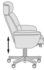
Gas lift seat height adjustment
