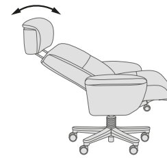
Manual height and angle adjustable headrest
